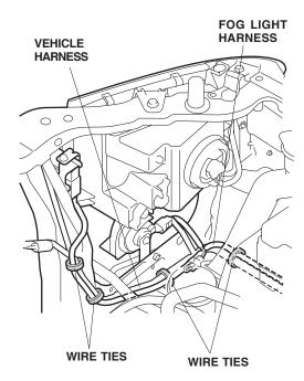
35. Secure the fog light harness to the vehicle harness with one wire tie. Secure the fog light harness to the right end of the bumper beam with one black wire tie with clip at the green tape.
