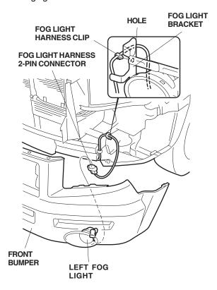
38. Reinstall the one clip, two bolts and two selftapping screws to secure the front bumper. Do not install the four outboard bolts to the front bumper at this time.
