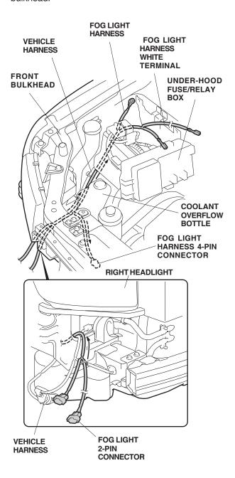
19. Route the white terminal from the fog light harness along the vehicle harness to the under-hood fuse/relay box.
