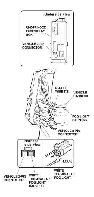
23. Unplug the vehicle 2-pin connector. Release the lock on the vehicle 2-pin connector, and push the fog light harness white terminal into the vehicle 2-pin connector. Reconnect the lock on the 2-pin connector, and plug the vehicle 2-pin connector into the under-hood fuse/relay box.
