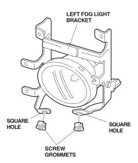
10. Attach the left fog light to the front bumper with two 5 x 16 mm self-tapping screws and two 5 x 12 mm self tapping screws (black).
