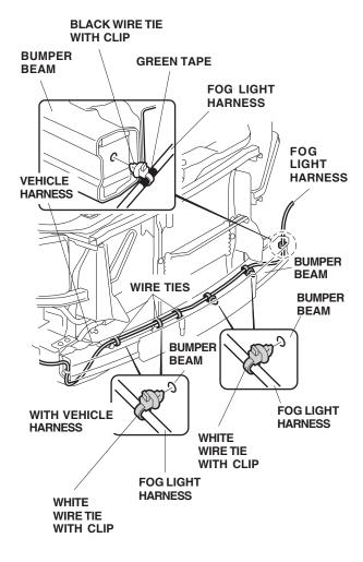
37. With an assistant holding the bumper near the vehicle, plug the fog light harness 2-pin connectors into the right and left fog light, and push the clip on the fog light harness into the hole of the right and left fog light bracket.
